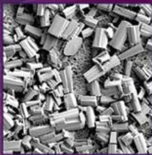
Wax crystals in Diesel fuel treated with Diesel Plus
