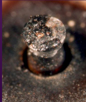
Injector pintle - a fuel system conditioner has not been used
